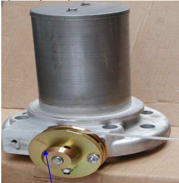
Wheel includes arrow indicator; when arrow is vertical valve is open, when horizontal valve is shut
